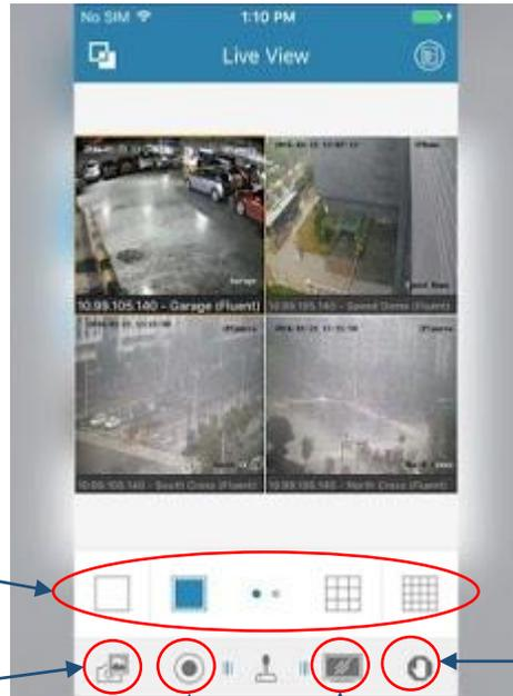
Select viewing options here. Select from single camera to 16 camera viewing.
